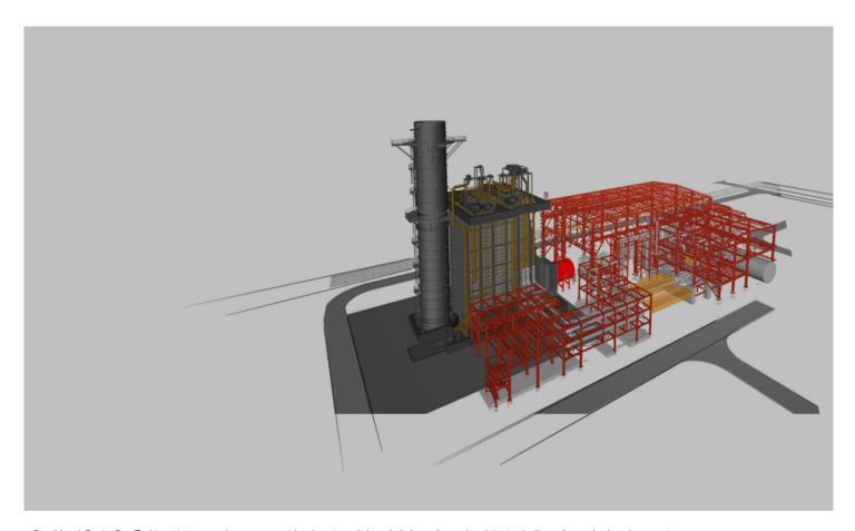
Combined Cycle Gas Turbine that comprises one combined cycle unit in a 1-1-1 configuration (single shaft configuration) and generates 840 MW. Located at the Industrial Area of Alexandroupolis (Greek), the Power Plant site has dimensions 349m by 222m including the boiler, turbine building (with the turbine pedestal inside) and the racks (main and secondary).
